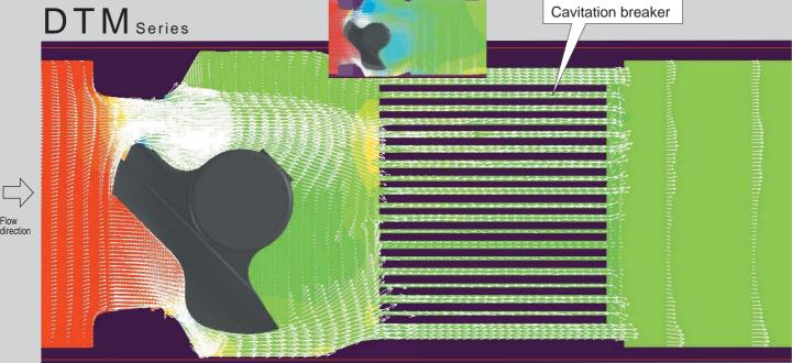
(Note) Colours show the pressure distribution. Red means a high pressure and blue means a low pressure.
